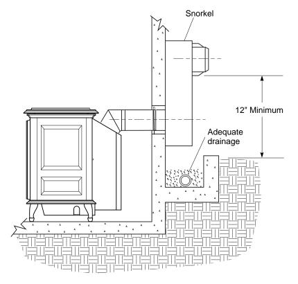
Figure 20 - Snorkel Termination with Drainage Pipe
